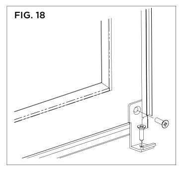
18. Find the location of the bottom bracket. Place the bottom wind stopper into the space between stationary panel and the sill tracks connected with bottom bracket. Bottom wind stopper to ensure its bottom fixed stably. Apply Silicone to fix the bottom wind stopper on the sill (Fig. 19 & 20)
