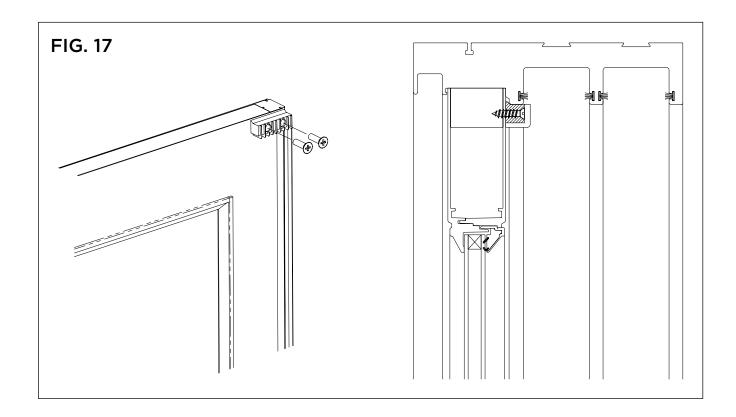
17. Secure the bottom bracket into the pre-drilled hole on the sill and stationary slab with #10x1" flathead screws. (Fig 18)
