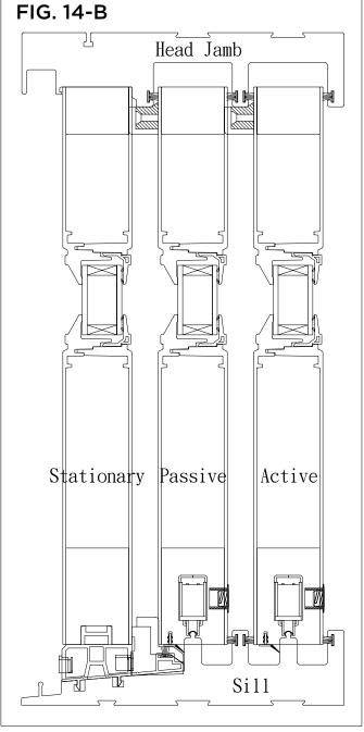
14. Unlock door and open active panel about half the width of the panel, remove active panel by lifting panel up and out from inner side. Make sure the Anti-lift block is parallel to the head jamb. (Fig. 15)
